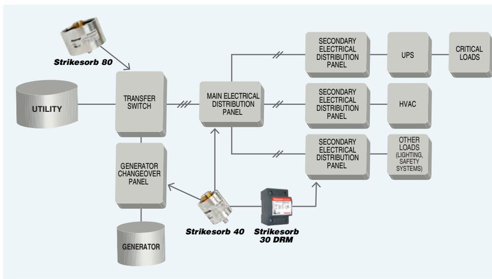
Figure 1: Recommended scheme for protection of critical systems
